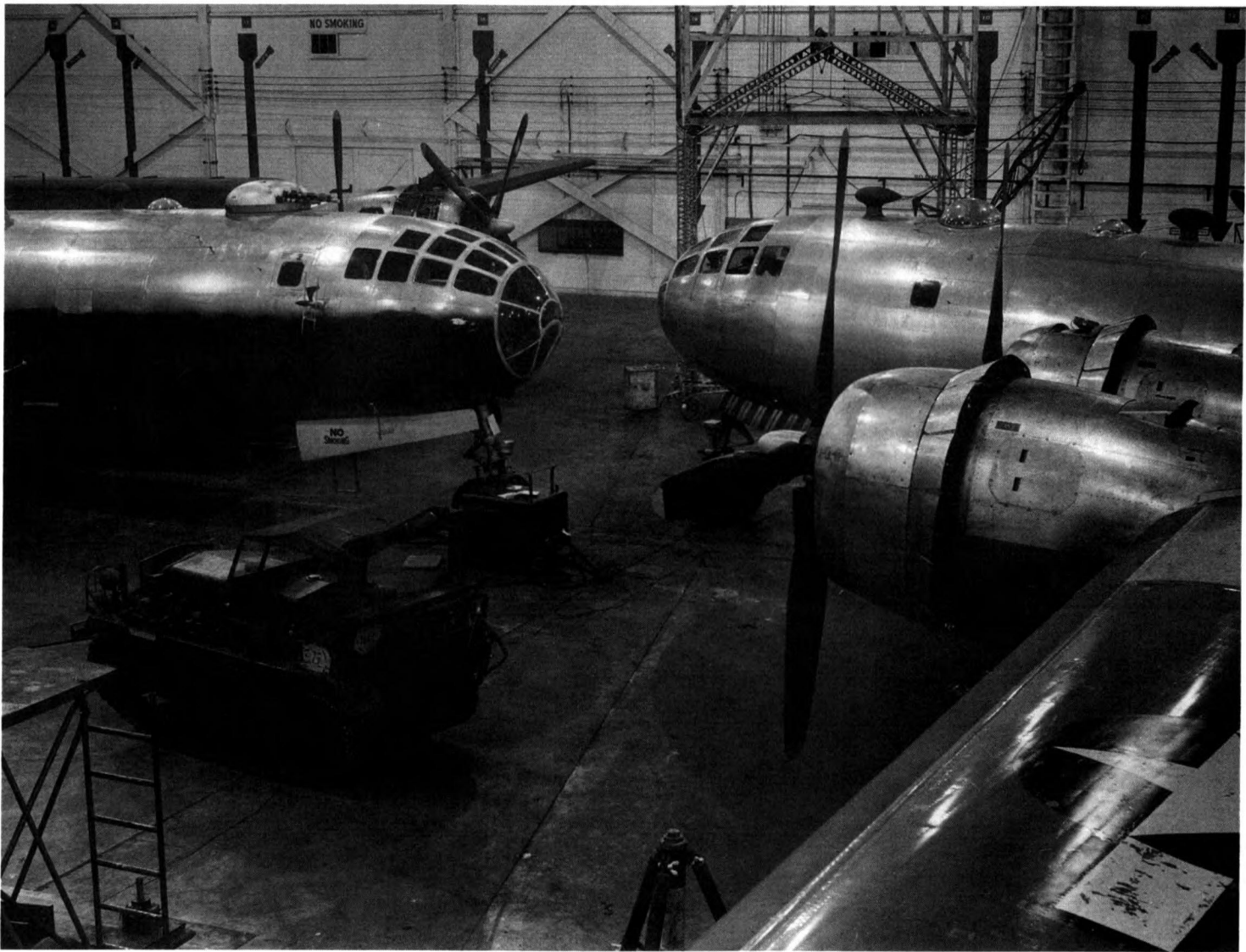
F-13s undergoing maintenance in Hangar No. 4. Left aircraft (with gun turrets) is partially modified. Right aircraft (with large astrodome) is more fully modified.
